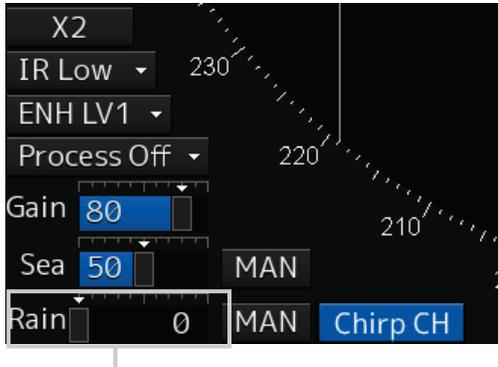
[Rain] (rain/snow clutter adjustment) slider
