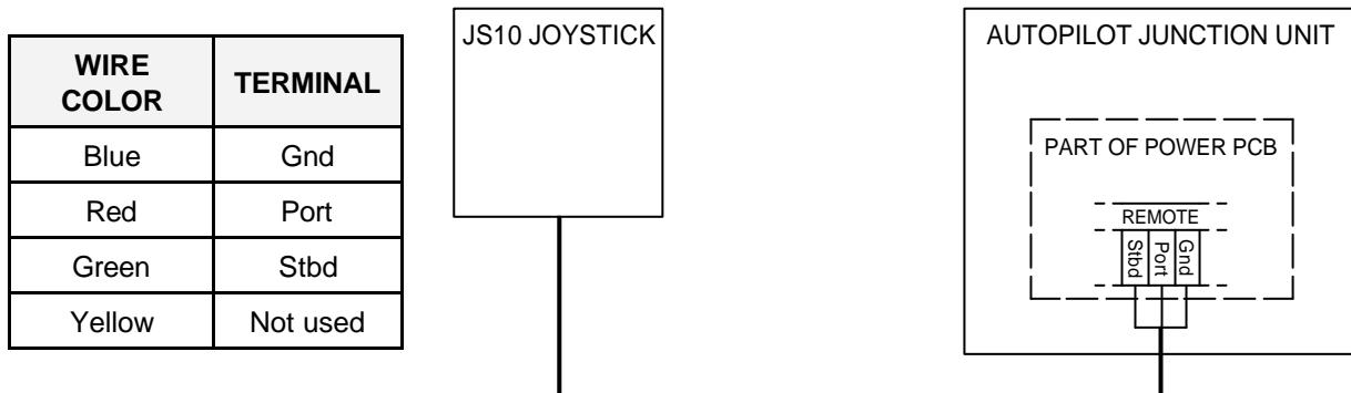
*Note: After installation, always check that correct direction of rudder movement is obtained. If not, reverse the red and the green wires!*
