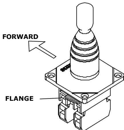
The joystick is anchored to the contact block by means of a snap-on flange. It should not be necessary to disconnect the joystick and the contact block for installation. If they have been disconnected, the joystick and the mounting plate have to be positioned into the contact block according to the drawing to get the correct port and starboard commands.
