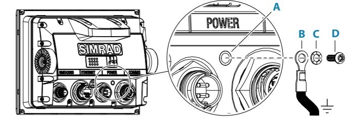
→ **Note:** It is recommended that the unit ground is connected to the vessel's bonded ground or a non-bonded RF ground.
